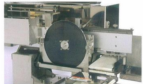
Covers around the blade can open/close easily when you do cleaning.
