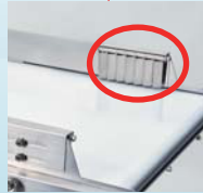
Added conveyor shooter prevents sliced meat dropping.
