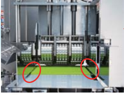
Newly added sensor in meat box to know the process ends.
