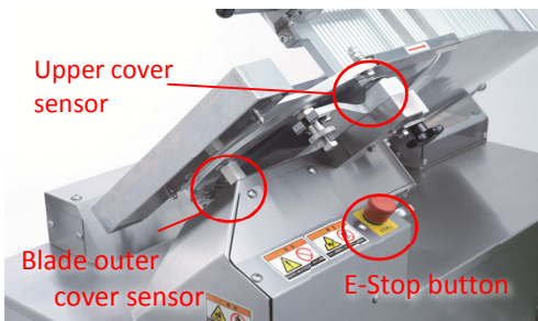
Enhanced safety by additional sensors and E-stop button.
