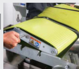
Easy detachment of the conveyor part
