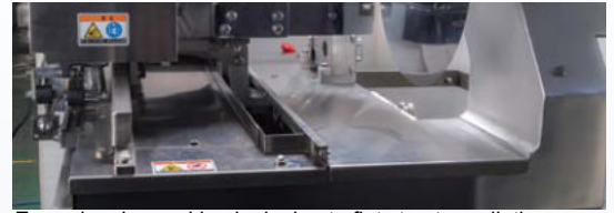
Easy cleaning and hygienic due to flat structure all the way to the back of the machine
