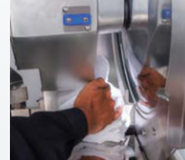
Space behind the round blade for easy cleaning
