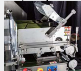
Resin parts are changed to stainless steel
