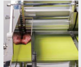
Minimum slicable ingredient width improved from 92mm to 70mm
