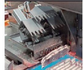
Counter plate pushes the remaining meat for a final slice to minimize the thickness of residual meat down to 15mm
