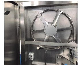
Automatically adjusts the tension of the blade and also has a load detection function
